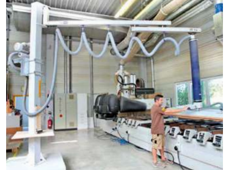
Telescopic jib for confined working areas
