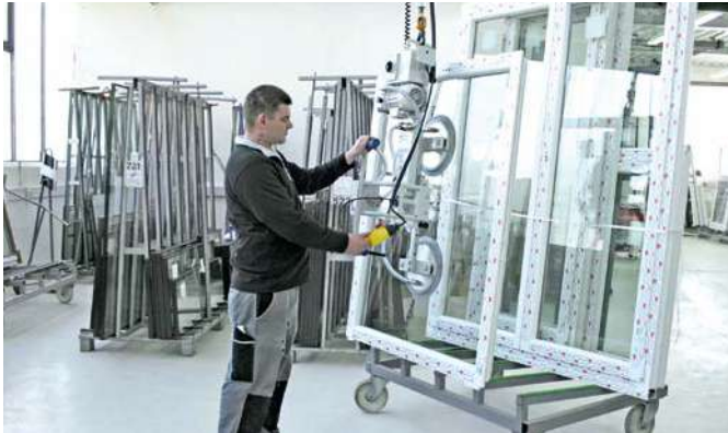
VacuMaster Window for rotating and palletizing windows
