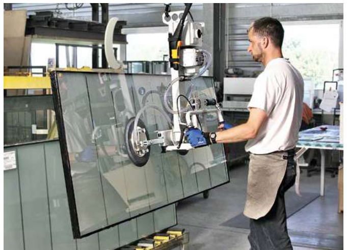
Vacuum lifting device VacuMaster Window for vertical handling of glass elements
