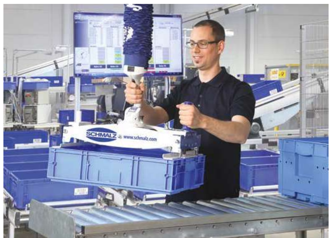
Vacuum tube lifter JumboFlex for handling transport and storage boxes
