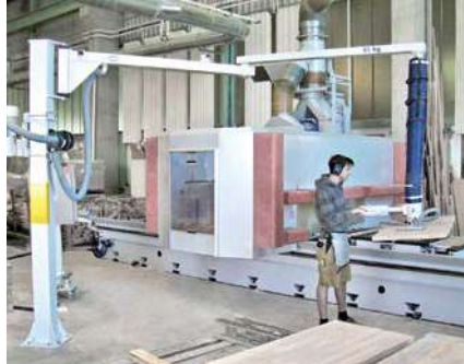
Articulated-arm jib to move around obstacles
