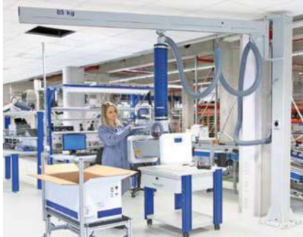
Flat jib for particularly low ceilings
